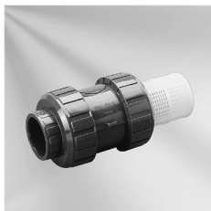
Fußventil S4 DN80 PVC grau PVC-U Klebemuffe d 4" ASTM PN6 EPDM EPDM Foot valve S4 DN80 PVC grey PVC-U solvent socket ends d 4" ASTM PN6 EPDM EPDM
