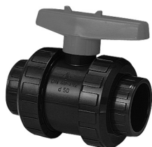
Kugelhahn S6 2W PVC grau PVC-U Klebemuffe ASTM PN16 FPM ptfе einzeln verpackt Ball Valve S6 2W PVC grey PVC-U solvent socket ends ASTM PN16 FPM ptfе single packed
