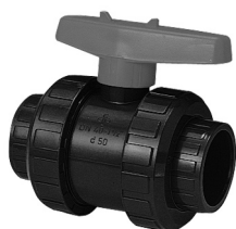
Kugelhahn S5 2W DN80 PVC grau PVC-U Klebemuffe d 4" ASTM PN6 EPDM PE Ball Valve S5 2W DN80 PVC grey PVC-U solvent socket ends d 4" ASTM PN6 EPDM PE
